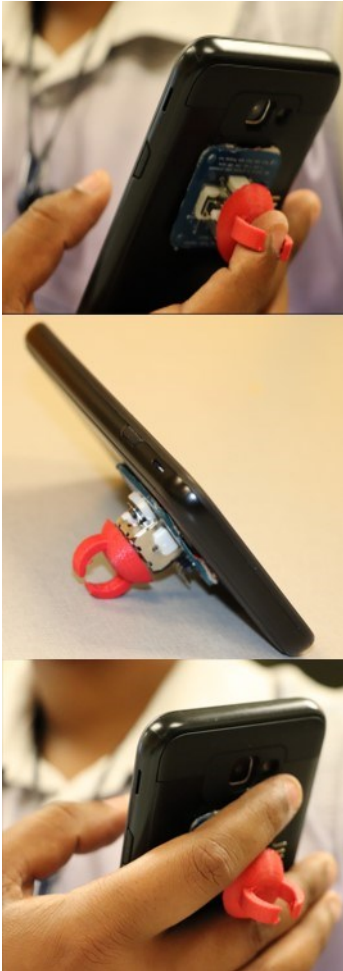
Figure 1. JoyHolder as back-of-device interaction (top), phone stand (center) and phone holder (bottom).
