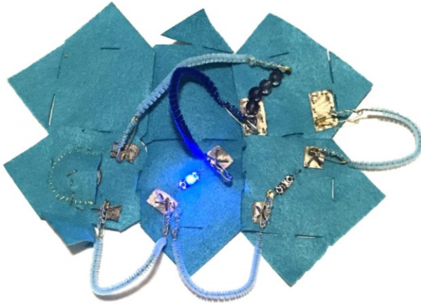
Figure 7—A simple circuit made with the medium-fidelity bits, including a tilt sensor that lights up.
