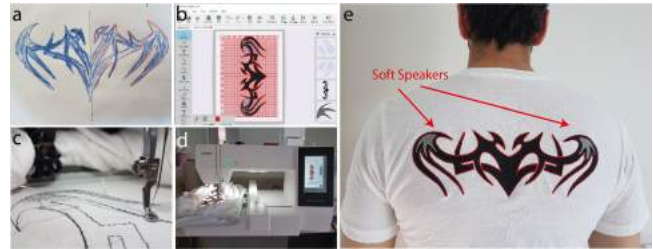
Figure 9: The making of the Tectonic-Tshirt: a) user sketch; b) pattern design; c) and d) digital-embroidery of Soft Speakers as part of the whole design; and e) wearing the t-shirt with Soft Speakers while gaming for personalized sounds and vibrations.
