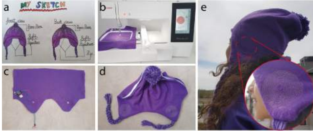
Figure 8: The making of the Talking-Tuque: a) Sketching the design; b) Digital embroidering Soft Speakers; c) Stitching the audio amplifier circuit to the fabric; d) Sewing the layers together with zippers and some embellishment; and e) The hat worn in winter on either face.
