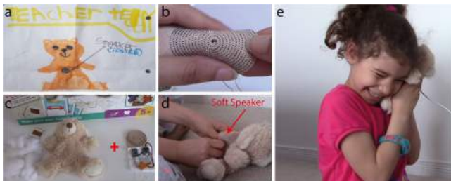
Figure 12: The making of Teacher-Teddy: a) Child sketch; b) Embroidering a Soft Speaker; c) Utilizing a DIY bear-making kit; d) Stuffing the circuit; e) e-learning with Teacher-Teddy.
