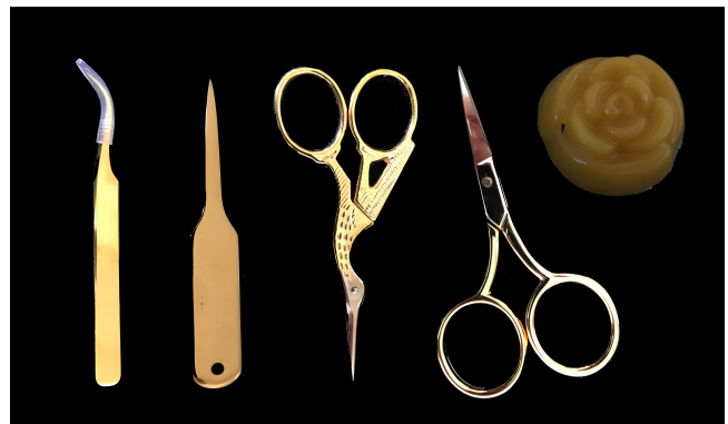
Figure 11: Common goldwork tools (from left to right): tweezers, mellor, embroidery scissors, goldwork scissors with serrated blade, beeswax.
