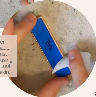
Copper tape is wrapped around the edges of the glass pieces.
