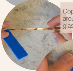
The copper edge is made flush against the glass using a smooth tool like a lathekin.
