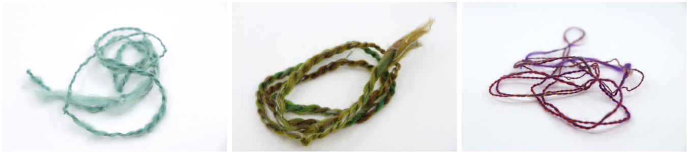
Figure 10: Participants created e-textile yarns that were conductive and could “blend” into textile projects.
