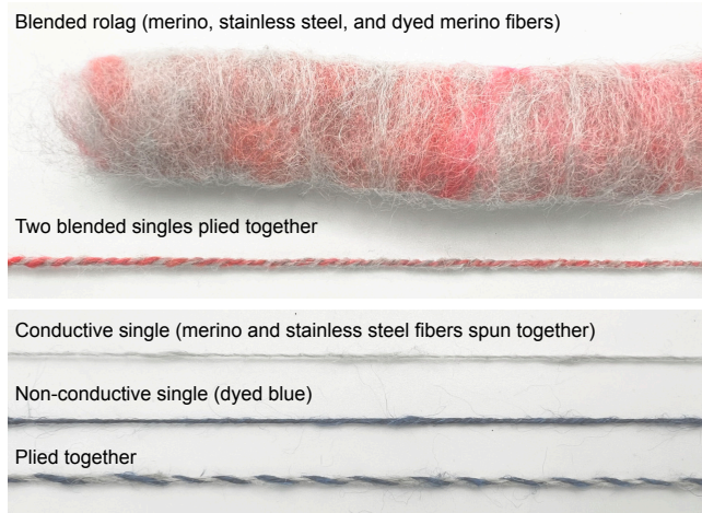
Figure 6: Hand-spun, conductive yarn can be created by blending fibers together (top) or by plying conductive and non-conductive singles together (bottom).
