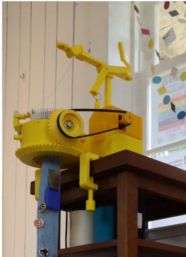
A. We replaced the hand crank with a motor.
