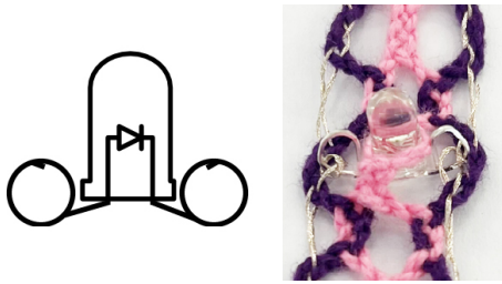
Figure 12: To transform LEDs into "beads" that could be laced, we curled up the LED's two "legs" into circular bead shapes. The smaller the circular hole, the better it held in place. Lace-makers recommended making the hole the same diameter as the thread or material you are using.
