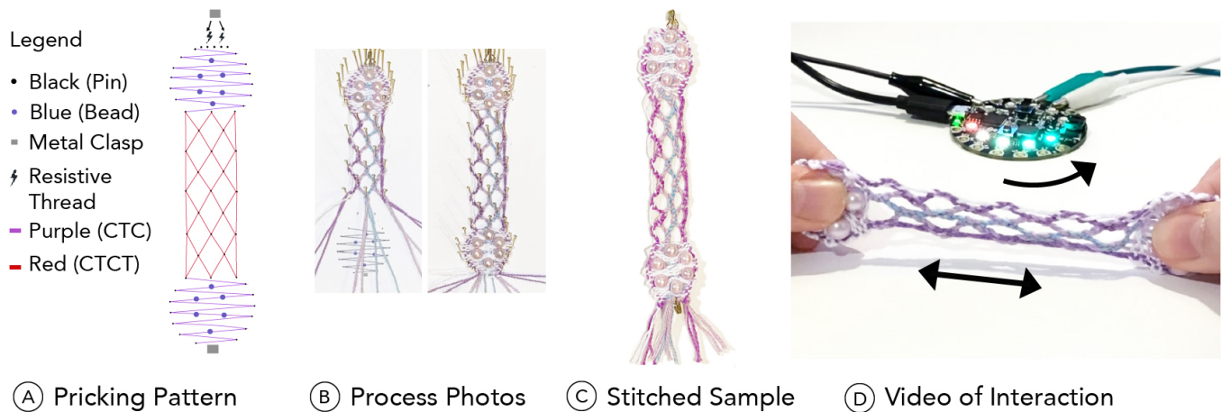
Figure 11: For each sample, we provided the following items for guild feedback: (a) bobbin lace patterns, (b) images with steps of the creation process, (c) photos of the final stitched sample, and (d) videos of the sample in action with an explanation of how it worked. This series shows the pattern, creation, and interaction of a bobbin lace stretch sensor with variable resistance thread.
