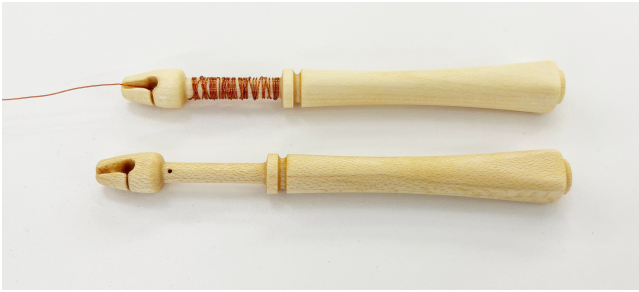
Figure 15: Bobbins designed by Richard Pikul for wire and gimp thread. The hole in the neck secures the wire for winding and the head holds and tensions it.
