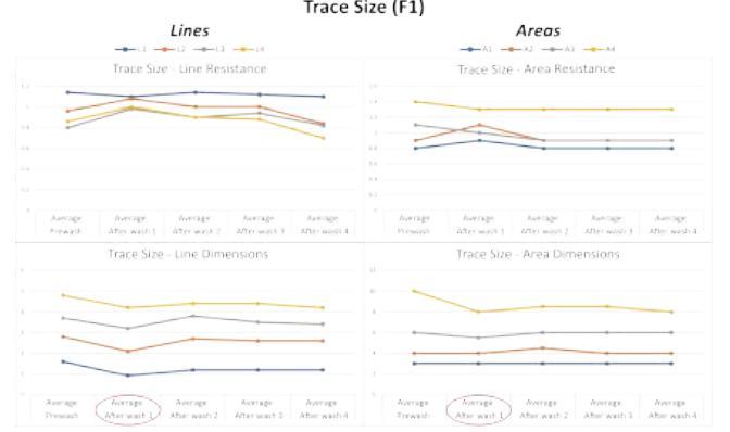
Figure 9: Washability Characterization: Trace size (F1) impact on resistance and dimensions (mm) after washing.
