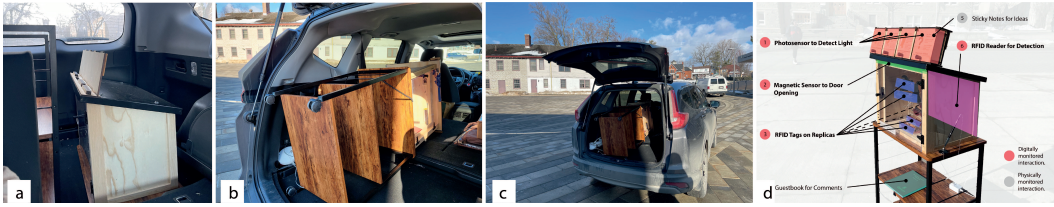
Fig. 4. Showing the MobileMuseum disassembled to fit upright in an SUV car (a) or alternatively placed fully assembled (b) inside the car (c), with all its interactive components (d).
