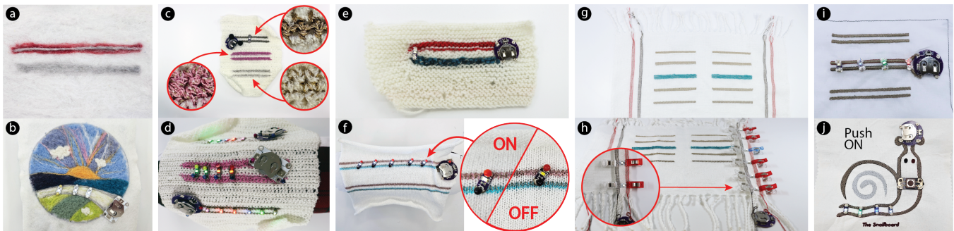
Figure 5: FabricBoard Demos: a) FeltBoard; b) with aesthetically rich design possibilities; c) CrochetBoard; d) with LEDs in a circuit connected using sewing pins; e) KnitBoard; f) with machine-knitting; g) WovenBoard resembling the solderless breadboard layout; h) an LED circuit connected to it using sewing clips; i) EmbroideredBoard; j) supporting creative shapes.
