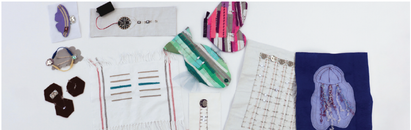
Figure 1: We explore the design of ‘FabricBoards’ for prototyping and testing wearable components using various textile crafts for creating FabricBoards through sewing, quilting, layering, weaving, knitting, felting, and embroidering.
