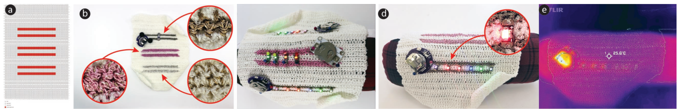
Figure 12: Designing the CrochetBoard: (a) on a digital stitch software (b) with 6 connection paths as 3 pairs of power/ground lines (c) that act as connection paths for up to (6x3) 18 LEDs (d) connected with magnets or sewing pins on an ironing cushion. (e) Thermal imaging shows the heatmap while powered by a 3V battery.
