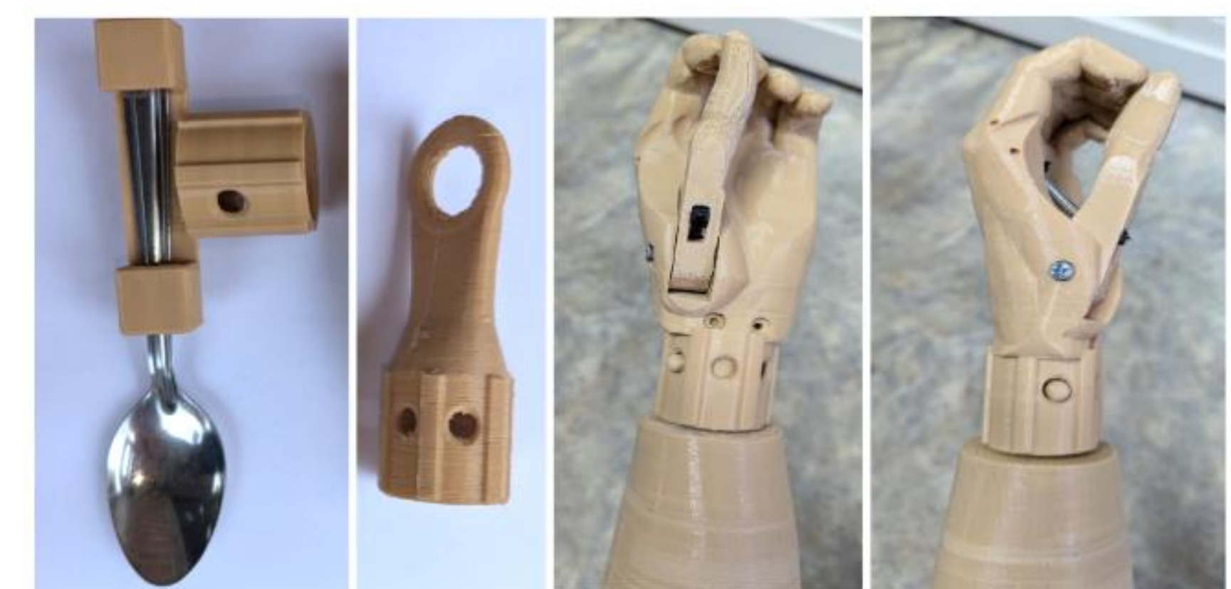
Fig. 2: Different hand attachments that are suitable for the arm with a 360 degrees rotation. Left to right: Utensil holder, bicycle attachment, gripper hand (neutral and 90 degrees rotation shown).
