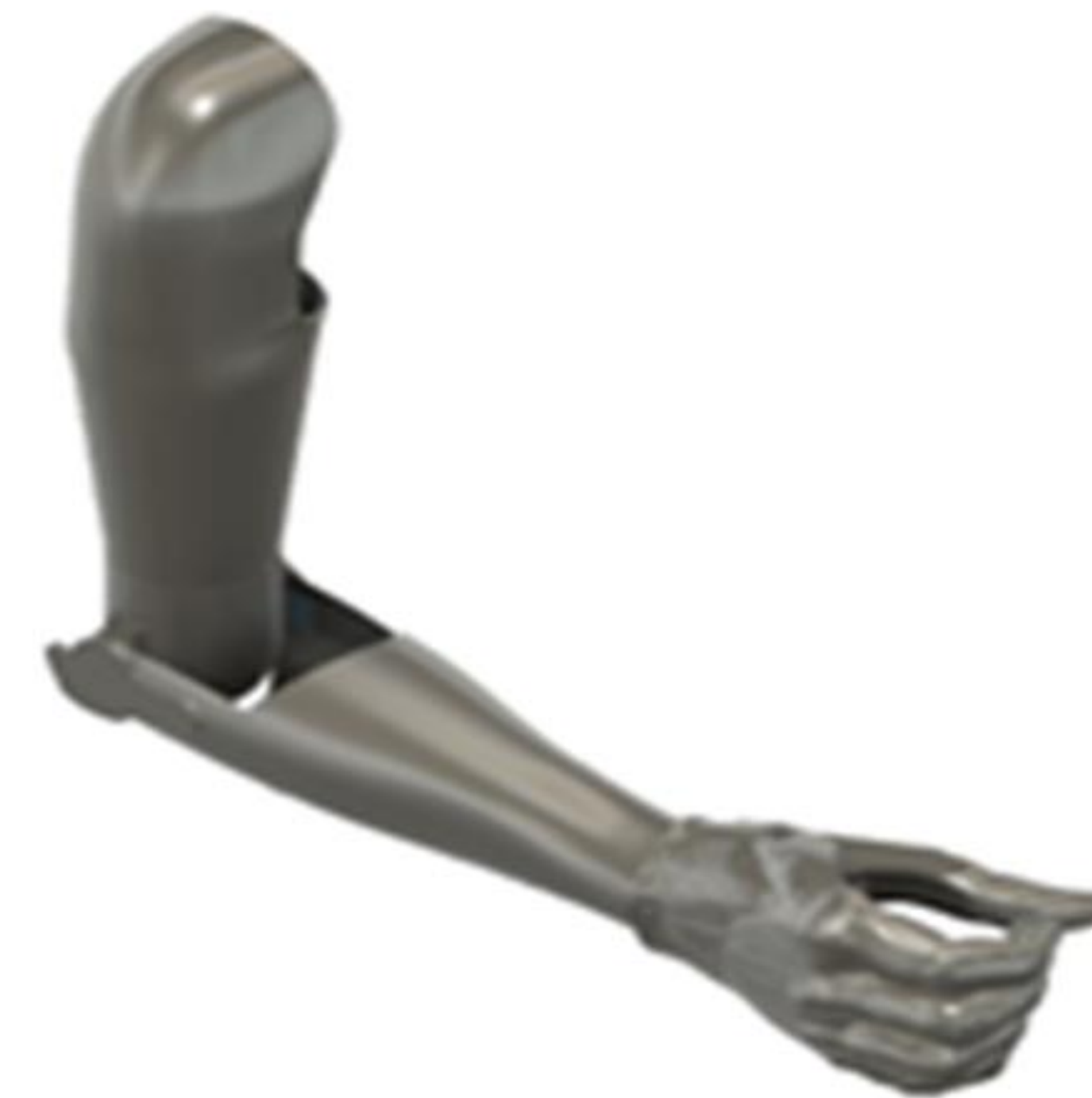
Fig. 2: CAD assembly of the shoulder, forearm and gripper hand prosthetic.
