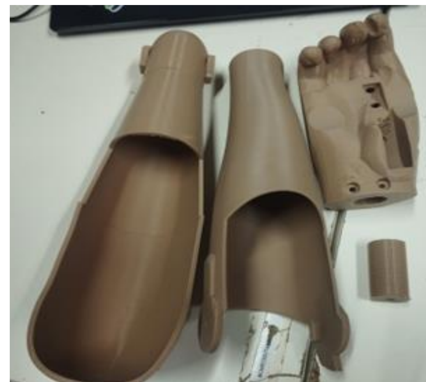
Fig. 3: A.R.M. Pieces include the arm, forearm, gripper hand, wrist bolt.
