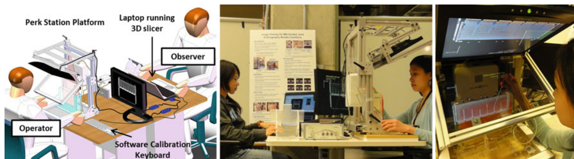
Fig. 9 Diagram of the experimental setup (left), the actual setup for freehand insertion (center), overlay insertion (right)
