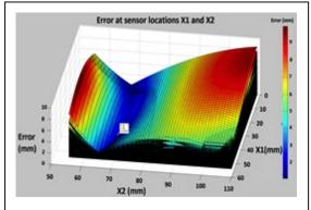
Fig. 2- "X" represents (x1, x2) optimal (45, 67) mm for maximum error of 0.61 mm
