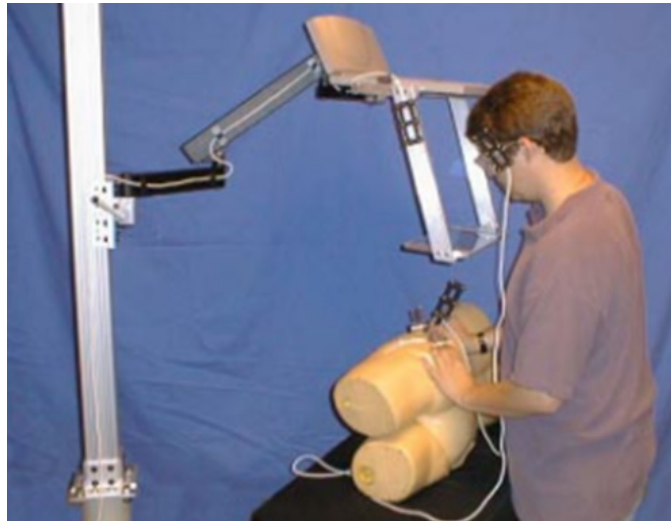
Figure 2.11: Volumetric image overlay prototype used for pelvic screw fixation simulation [15]. The physician's head is continuously tracked.
