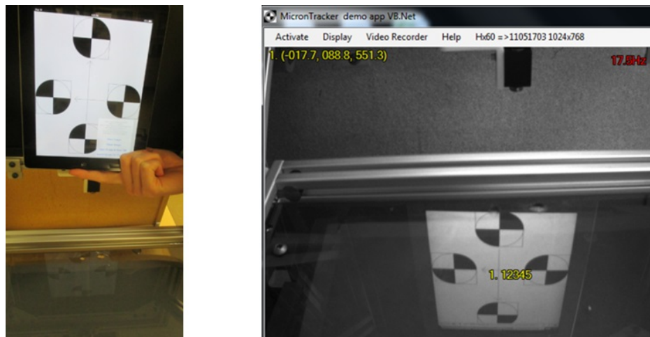
Figure 4.7: Tablet display device (iPad2) feasibility study: Left) Marker displayed upon iPad2 device. Right) Pose of the virtual reflected marker determined by MicronTracker.
