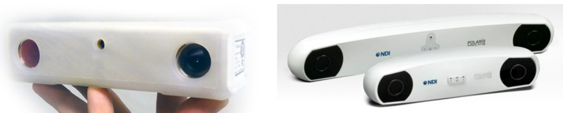
Figure 3.18: Optical tracking systems: A) MicronTracker ( Claron Technology Inc. ). B) Polaris Tracker ( NDI Medical Inc. ).
