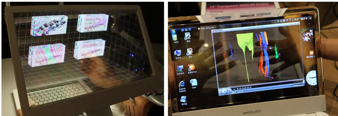
Figure 5.9: SpaceTop: Integrating 2D and spatial 3D Interactions in a see through desktop environment. ( Microsoft Research, Applied Sciences Group )
