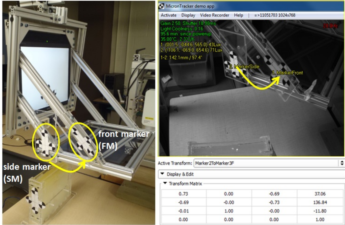
Figure 3.24: Auto-direct calibration Step 2: Left) Transform ( {}^{SM}T_{FM} ) \Rightarrow side marker (SM) to front marker (MF). Right-top) MicronTracker camera image indicating markers' pose. Right-bottom) Transform obtained using the "Transform recorder" Perk Tutor module of 3D Slicer.
