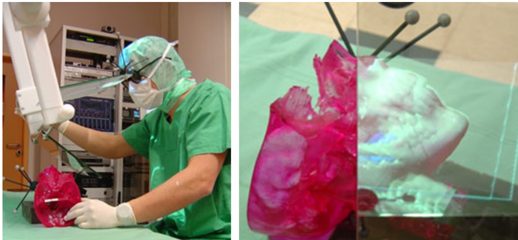
Figure 2.12: ARSyS-Tricorder : Image overlay system with a large screen for interventional image guidance ( Fraunhofer Institut Intelligente Analyse und Informationssysteme (IAIS), Sankt Augustin, Germany )
