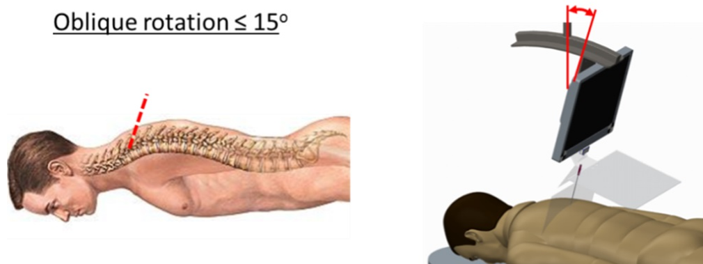
Figure 3.8: Viewbox rotation about the RCM for oblique rotation of \leq \pm 15^\circ .
