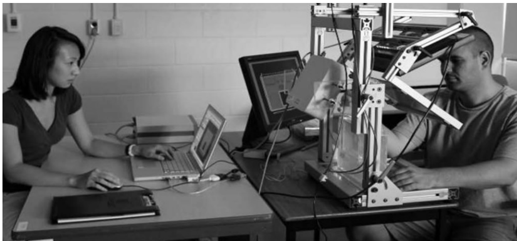
Figure 2.17: Perk Station [18]: The observer (left) sits opposite the trainee (right) and monitors the needle insertion visually. The side of the phantom facing the trainee is covered to prevent the trainee from direct visual access to the target.
