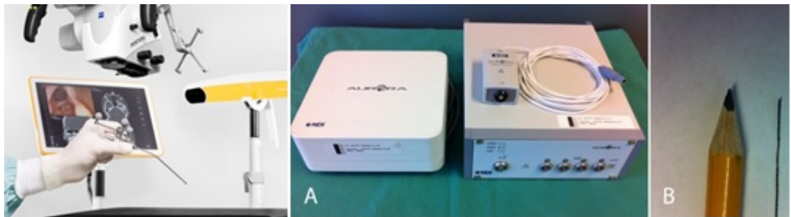
Figure 2.1: Left) Optical navigation system ( BrainLab AG ). Right) A) Electromagnetic tracking system - NDI Aurora NDI Medical Inc. . B) Tracking sensor 0.5 mm dia [6].
