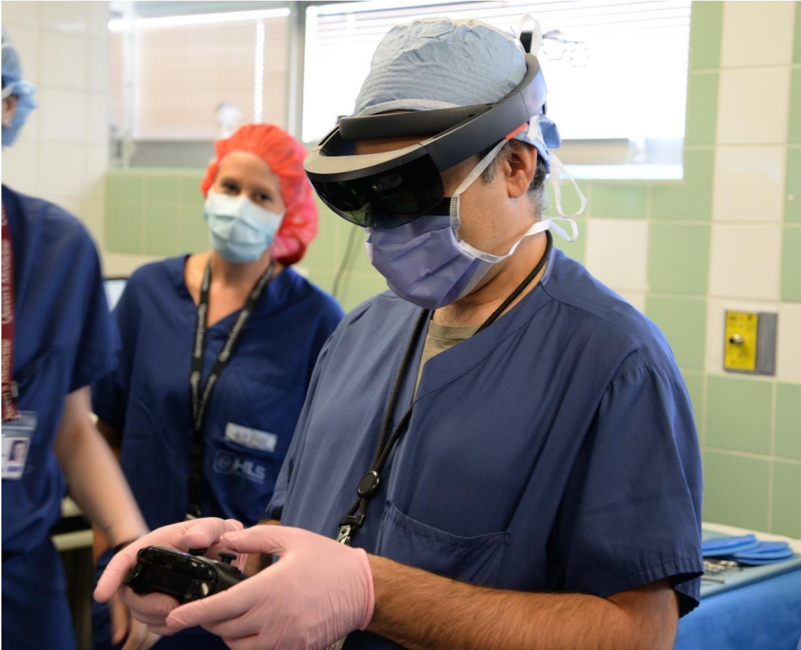
Figure 16. Neurosurgeon using the Xbox One Wireless Controller while wearing the HoloLens to register the holographic models to a patient.
