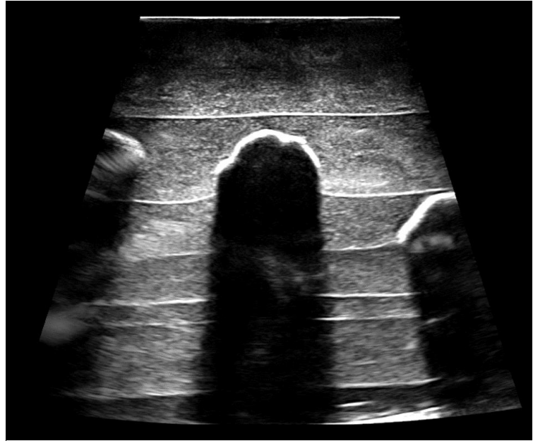
Figure 13: Parasagittal ultrasound image of a phantom model's transverse processes
