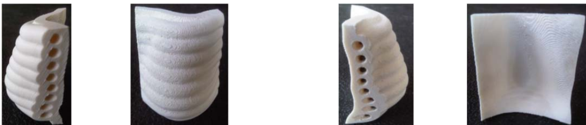
Figure 4: The 3D printed from ABS Plus plastic material surface mould applicator of the nose region of the inhouse wax head phantom
