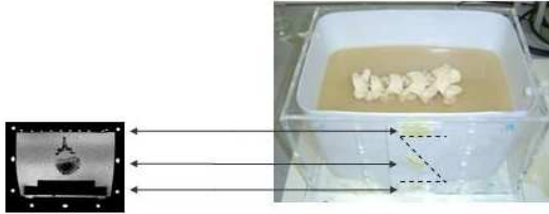
Figure 3. Phantom design showing spine partially embedded in gel and fiducial markers both on the phantom and their corresponding MR image.
