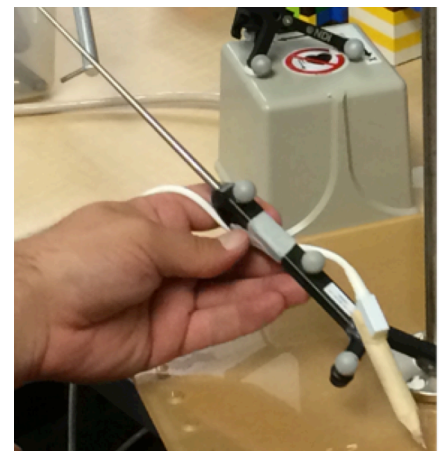
Figure 1. Hot glue was used in order to attach the Ascension's EM sensor to the optical pointer. The EM sensor is attached to a pencil serving as a modified tip which is itself attached to the pointer.
