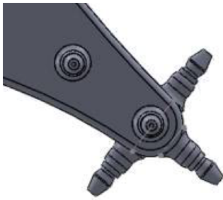
Figure 4. A zoomed-in image of the dual-modality pointer showing the multiple pegs available for the attachment of optical markers.
