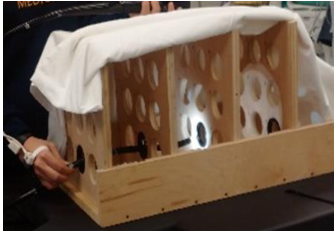
1 2 Fig. 5. Close-up view of the wooden bench-top model. The black rings indicate the holes through 3 which the operator must navigate the colonoscope.
