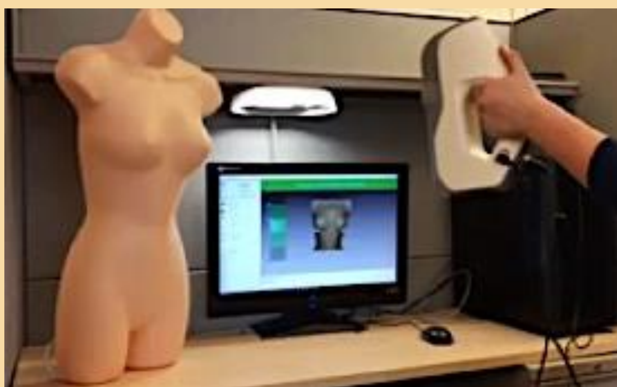
Fig 3. Female mannequin scanned with Artec Eva
