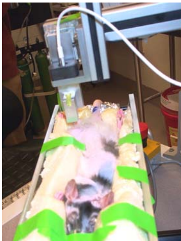
Fig. 3. Oxylite probe inserted in rodent
