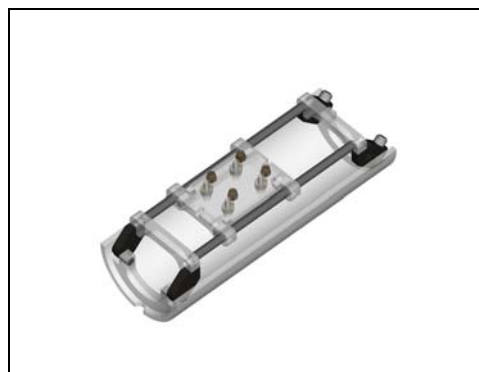
Fig. 4. Rodent bed with fiducial bridge
