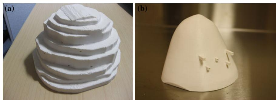
**Fig. 6** Templates created using 3D rapid prototype printer *Left a* first template designed and printed for catheter guidance. *Right b* template printed during second round of experimentation with improvements to template made
