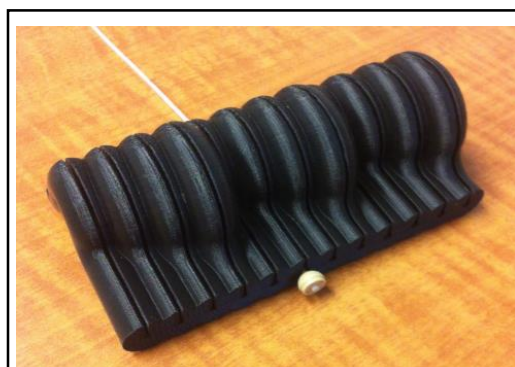
Fig. 2. Calibration object to determine optimal channel dimensions
