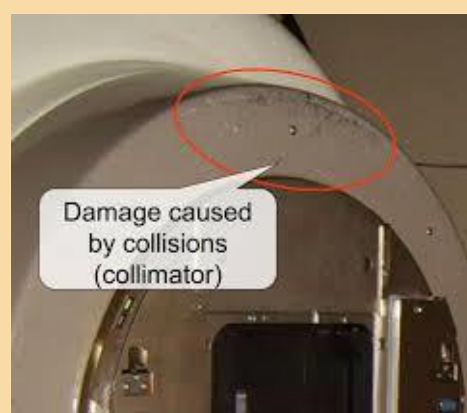
Figure 3. Collimator damage caused by collisions with other parts of linac.
