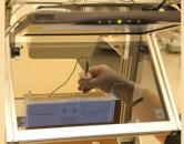
Experiments were carried out using the PerkStation hardware and software system. The needle was tracked by an NDI Aurora (NDI, Waterloo, ON, Canada) electromagnetic measurement system, and its trajectory was recorded for off-line analysis.
