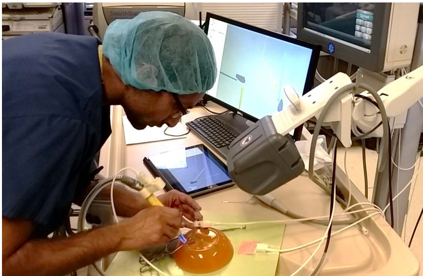
Figure 1. Experiment for testing of the intraoperative user interface on plastic phantoms.
