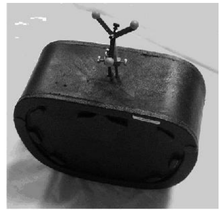
Figure 4: Interventional phantom with fiducial carrier
