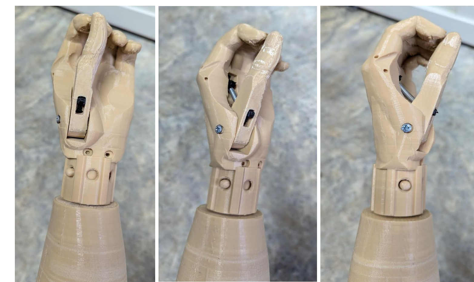
Fig. 2: 360 degrees rotation of the gripper hand attachment (90 degrees shown).
