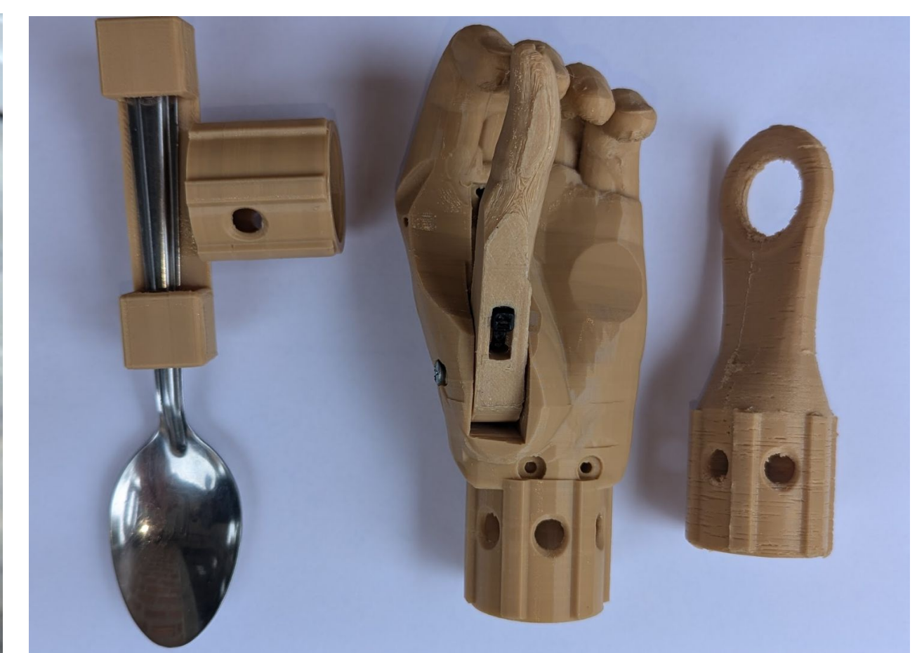
Fig. 3: Different hand attachments that are suitable for the arm.
